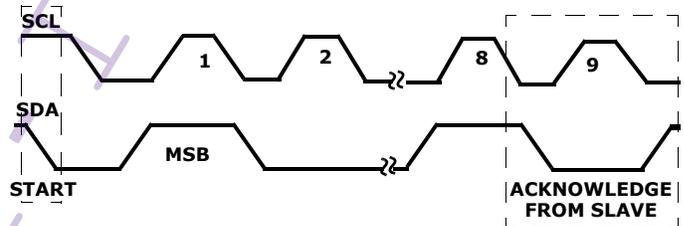
FIGURE 19. ACKNOWLEDGE ON THE I<sup>2</sup>C BUS
