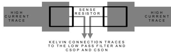
FIGURE 28. CURRENT SENSE RESISTOR LAYOUT
