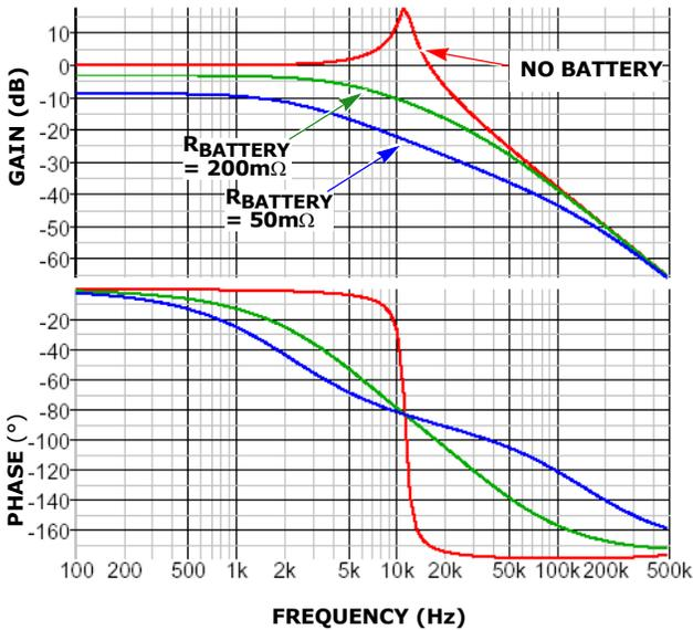
FIGURE 26. FREQUENCY RESPONSE OF THE LC OUTPUT FILTER
