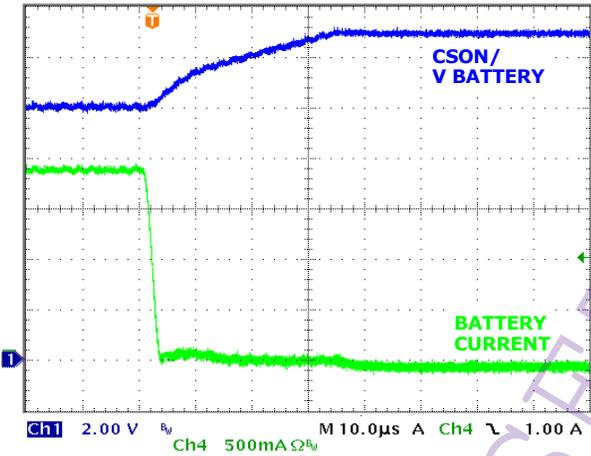
FIGURE 13. BATTERY REMOVAL
