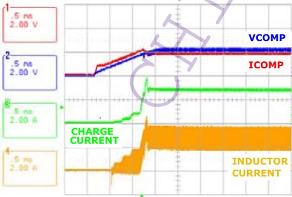
FIGURE 9. CHARGE ENABLE
