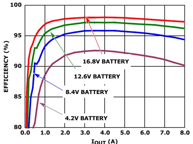
**FIGURE 2. EFFICIENCY vs CHARGE CURRENT AND BATTERY VOLTAGE**
